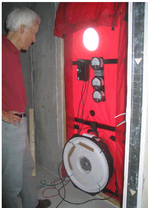
Fig. 7.1.1.: Blower Door test in an apartment.
