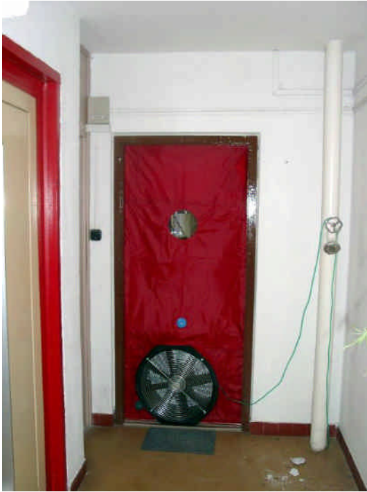
Fig. 8.6.1. Illustration of Blowerdoor test in Solanova demonstration project in Hungary.
