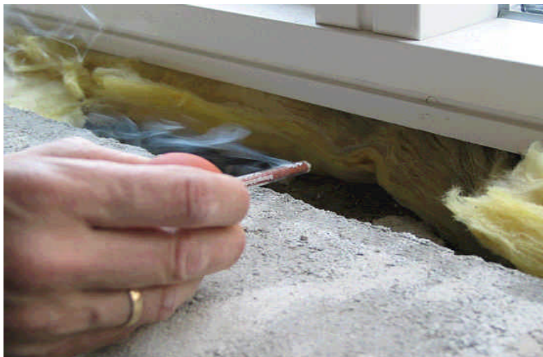
Fig. 7.1.2.: Example of registration of white smoke movement to trace cracks and crevices in combination with the blower door test.
